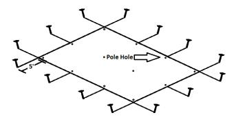
At the end of each rope, there are rope slides that make a loop. Place the loop around all of the stakes and leave them loose.
