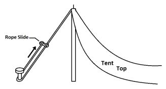
With all 4 corners up, take the center poles and place it in the holes in the peak and push up until they are both straight up and down. Place the remaining white poles around the tent and tighten with the rope slides.
