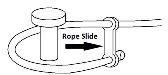
Start at one corner and insert the tip of the pole into the pole hole. (A pole hole is shown in the 1st image). Raise the pole until it is upright and tighten both ropes by pulling the rope slides upward. Continue with all 4 corners. Only the corners will have 2 ropes to tighten.
